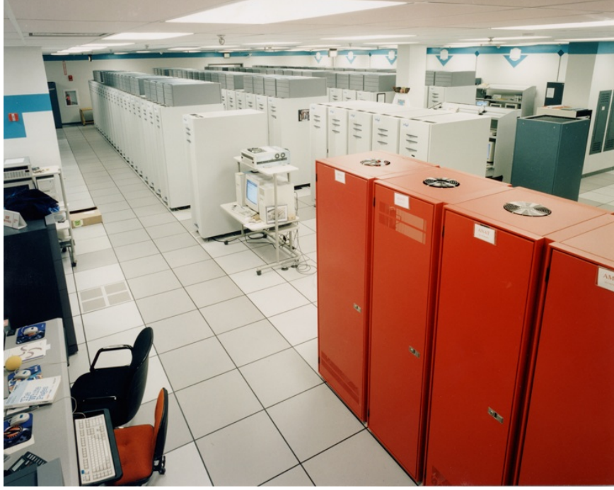
Figure 2.2: ASCI Red consisted of 104 cabinets, taking up about 2,500 square feet in the Sandia National Laboratories.
