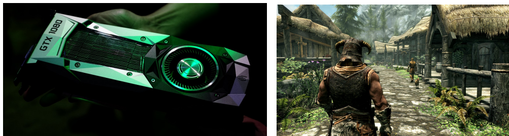
Figure 2.4: The Nvidia GTX 1080 was launched in 2016, supporting 2560 CUDA cores. Most modern user oriented CPUs have 4 to 8 computing cores [18]. These cards are marketed and mostly used for video games and graphics applications but are increasingly being used for optimized general and scientific programming.
