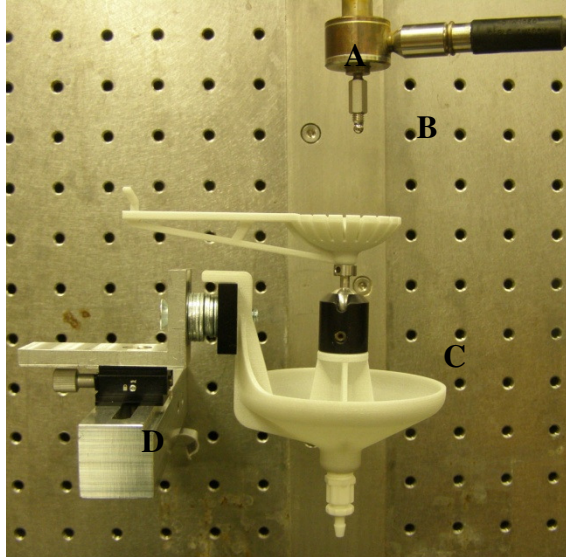
Fig 3- 1: Macro-indentation setup showing: A) load cell, B) spherical indenter and set screw, C) custom-articulating drainage platform, D) 2-axis manual positioner
