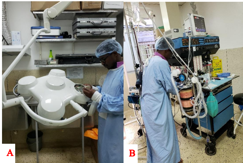
Figure 1: A) Engineer repairing light fixture in endoscopy room B) Engineer repairing bellows of ventilator in Theatre
